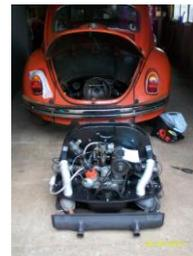
Whilst sorting the oil leak we thought we would tidy up Emily's tin wear, the fan housing was full of grease and dirt! After a clean and paint the tin wear looked good and it was time to refit it, now I hope I can remember how it all fits!
